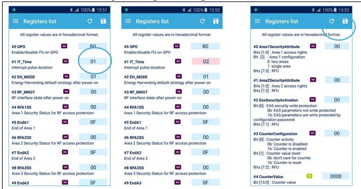
Figure 26. Registers management screens
